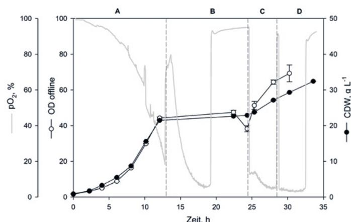
Fig. 4: Process overview of the batch/pulse method showing biomass growth on glucose (phase A, 0 to 13 h) and subsequent induction via MeOH pulses (phases B-D, 1% v/v).
