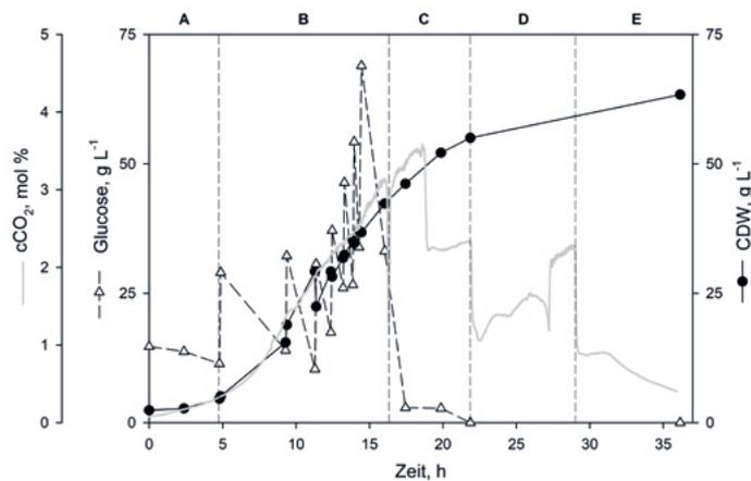
Fig. 5: Process overview of the semi-continuous feed method for biomass formation on 60 g L<sup>-1</sup>. Repeated glucose pulses (phase B) for testing substrate inhibition. Process phases separated by vertical dotted lines.
