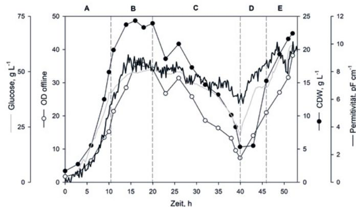
Fig. 7: Comparison between online biomass-monitoring sensors in the Minifors 2 during continuous cultivation (see Fig. 6 for additional process parameters).
