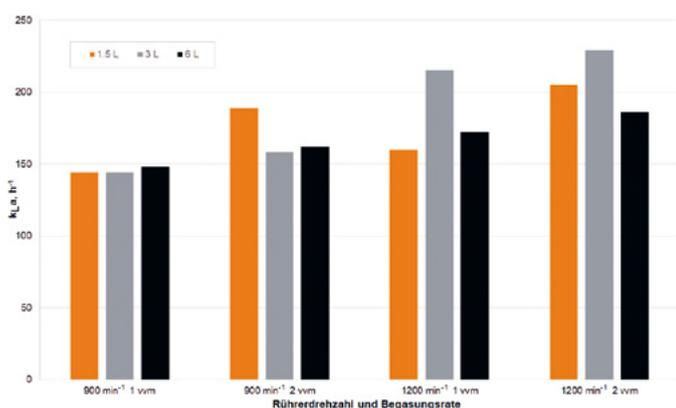
Fig. 2:  $k_L a$  values for the Minifors 2 at 900 and 1200 min<sup>-1</sup> and 1 and 2 vvm.
