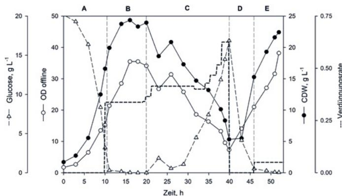
Fig. 6: Process overview of the continuous method. An initial batch phase (A) was followed by a phase with a constant dilution rate (B), a phase with a controlled elution step (C), a biomass re-enrichment phase (D), and a phase focused on product formation (E).
