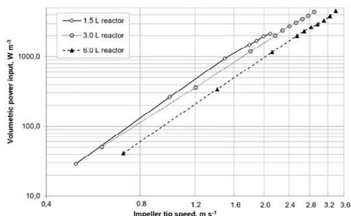
Fig. 3: Volumetric power input (in W m<sup>-3</sup>) for all three reactors at different impeller tip speeds (in m s<sup>-1</sup>) and maximum working volume.
